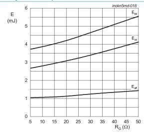
$I_{C}$  = 50 A;  $V_{GE}$  = 15V/0V;  $T_{j}$  = 150 °C;  $V_{CE}$  = 400 V; inductive load
