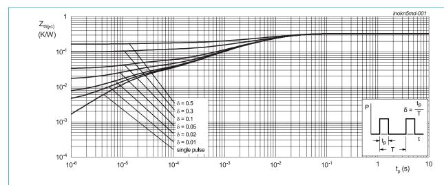
Fig. 1. Transient thermal impedance from junction to case as a function of pulse duration; IGBT
