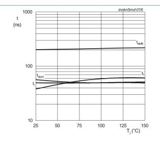
$I_C = 50 \text{ A}; V_{GE} = 15 \text{V/0V}; R_q = 10 \Omega;$
