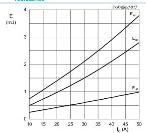
$R_g$  = 10  $\Omega$ ;  $V_{GE}$  = 15V/0V;  $T_j$  = 150 °C;  $V_{CE}$  = 400 V; inductive load
