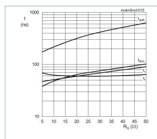
$\rm I_{C}$  = 50 A;  $\rm V_{GE}$  = 15V/0V;  $\rm T_{j}$  = 150 °C;  $\rm V_{CE}$  = 400 V; inductive load
